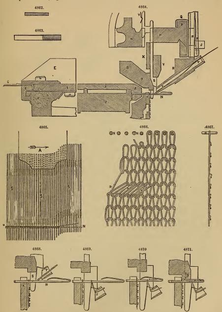
through which the sinkers slide, the walls of these grooves press the points of the beards of the needles into the grooves in their stems, as seen in Fig. 4871, and dotted in Fig. 4859. The needles then retire still farther, the new loops being still round the stems and under the beards of the needles, while the old loops now slide over the beards, as in Fig. 4872, and the presser-bar B is raised again as soon as the points of the beards have fairly entered the old loops on the needles,
